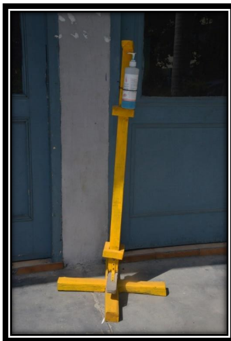
Waste Wood Used to Make Sanitizer Dispenser.
